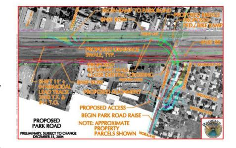
the new mainline track added on the south side of the rail corridor. Ramps would be constructed to accommodate traffic connecting to Park Road or SR 290 (Trent Avenue) to avoid major modifications to Trent Avenue.
